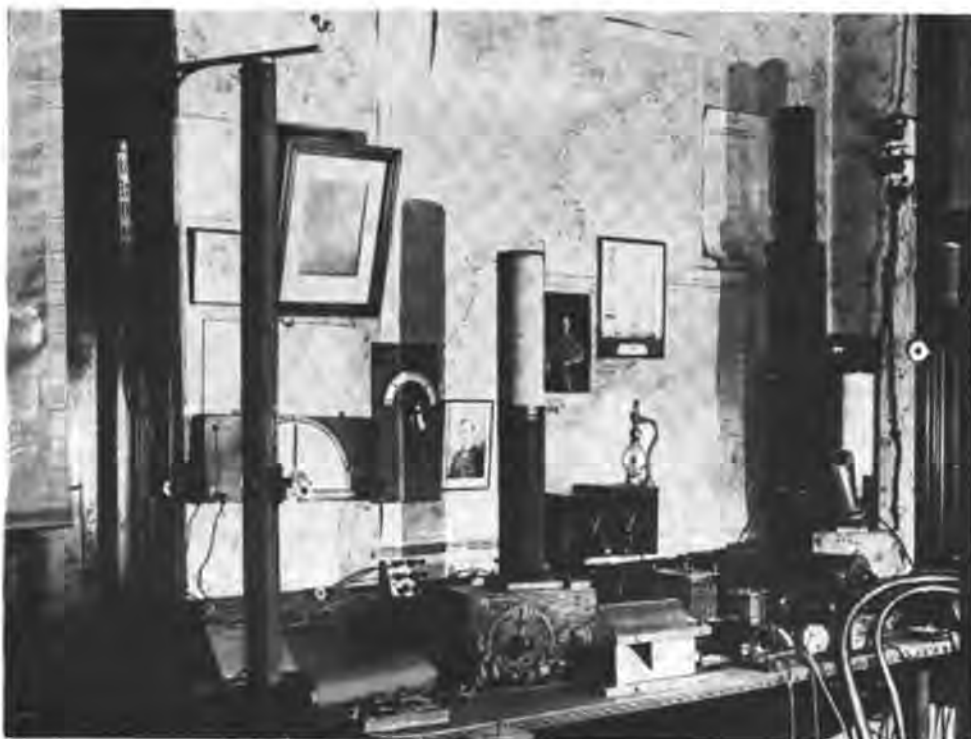
The amateur station of Charles Apgar. Equipment with which the Sayville wireless messages were recorded
